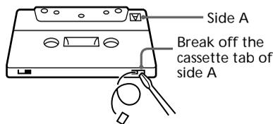
If you later want to reuse the tape for recording, cover the broken tab with adhesive tape. However, be careful not to cover the detector slots which allow the tape player to automatically detect the type of tape.
