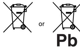
On certain batteries this symbol might be used in combination with a chemical symbol. The chemical symbols for mercury (Hg) or lead (Pb) are added if the battery contains more than 0.0005% mercury or 0.004% lead.
