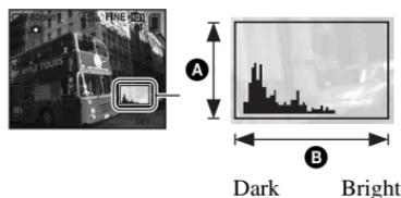
A histogram is a graph showing the brightness of an image. Set the mode switch to in advance, then press repeatedly to display the histogram. The graph display indicates a bright image when skewed to the right side, a dark image when skewed to the left side. A histogram can be used to check the exposure and adjust [EV].
