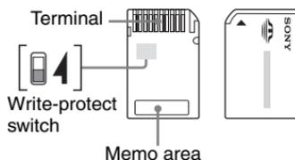
The position and/or the shape of the write-protect switch<sup>\*4</sup> may differ depending on the “Memory Stick Duo” you use.
