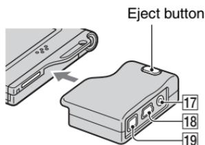
To detach the Interface Adaptor, hold down the eject button as you remove the Interface Adaptor.
